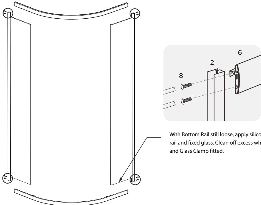
With Bottom Rail still loose, apply silicone between rail and fixed glass. Clean off excess when frame is tight, and Glass Clamp fitted.
